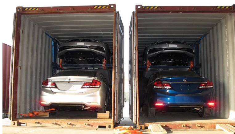
Figure 69: Rack and Cassette Systems for Loading of Cars in Containers
