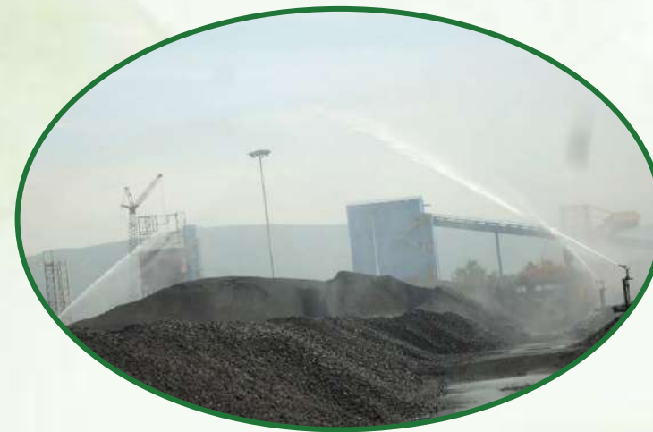
Treated Water From 10 MLD STP, Being Used For Dust Suppression
