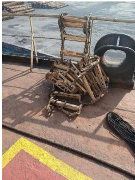
Poor condition and improper securing of pilot ladder
