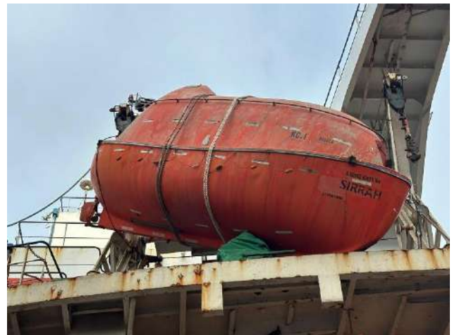
Lifeboat stowed with Uprooted Hook
