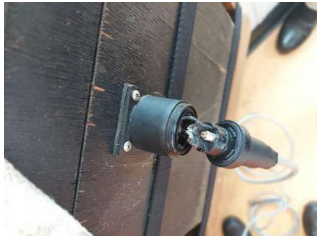
Aldis Lamp Socket damaged
