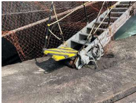
Damaged Gangway Rollers
