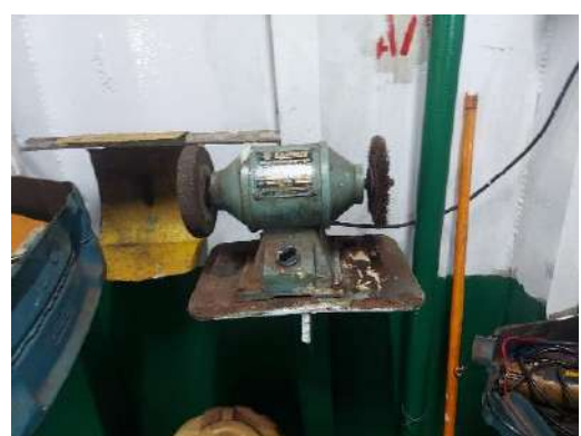
Safety Guards missing in Grinding Machine
