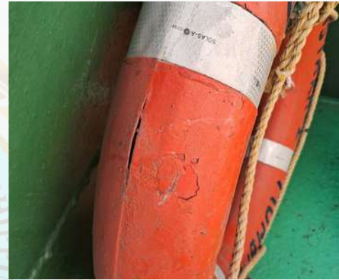
Cracked and holded lifebuoys
